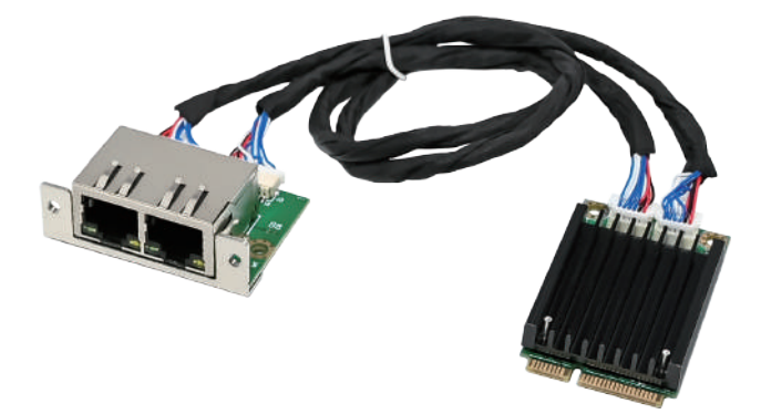
RJ45 Board: L45 x W30 x H15 mm
