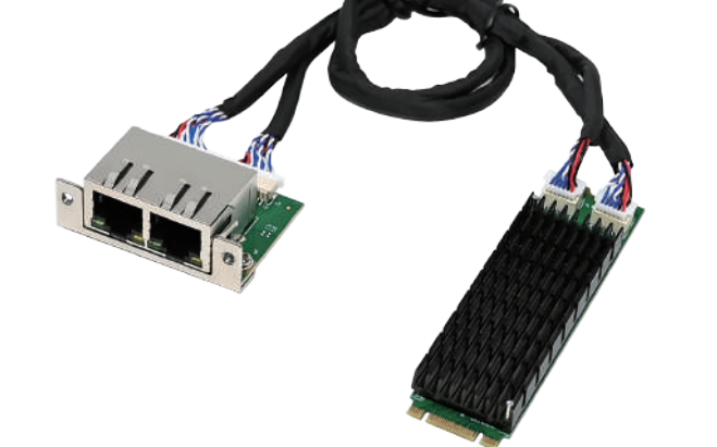
RJ45 Board: L30 x W33 x H15 mm
